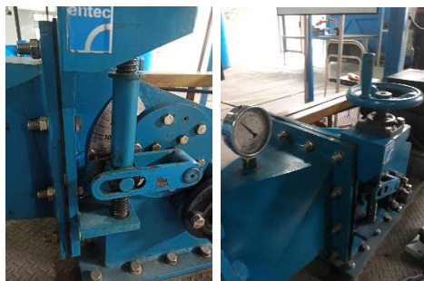
Gambar 4. Tuas guide vanes ( \alpha^0 )
